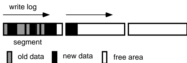
Figure 9: Segments in Log-Structured File System
